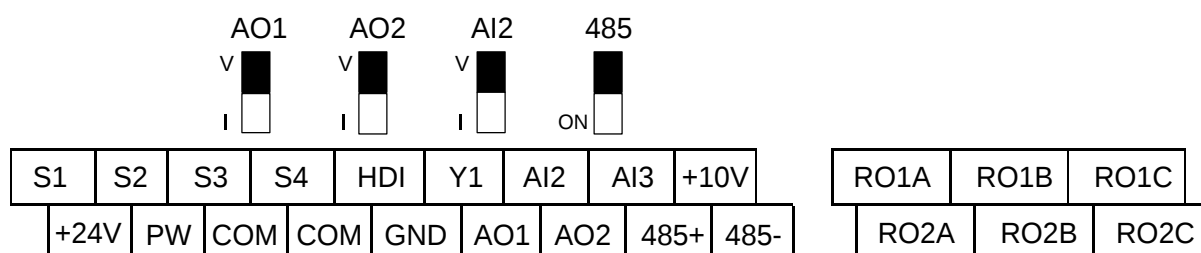
Figure 3–2 Control circuit terminal diagram for 4kW and higher inverters
